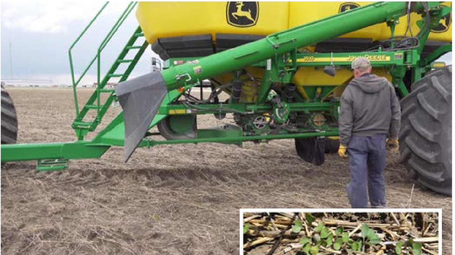
Above: Calibrating a John Deere seeder to apply varying rates of treated and untreated seed for a field trial on flea beetles and seed treatment insecticides.
