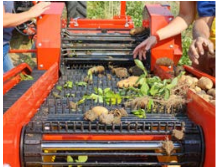
Harvest crew keeps up with potatoes as they move along the two primary tracks to separate the spud from the soil. Taken during the first test run of the new harvester in a trial for Farming Smarter's russet potato fertility project, September 2024. PHOTO: FARMING SMARTER
