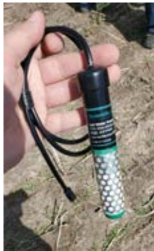
One of the sensors used in our Monitoring Soil Moisture project. Multiple sensors are placed at one location at various depths.
