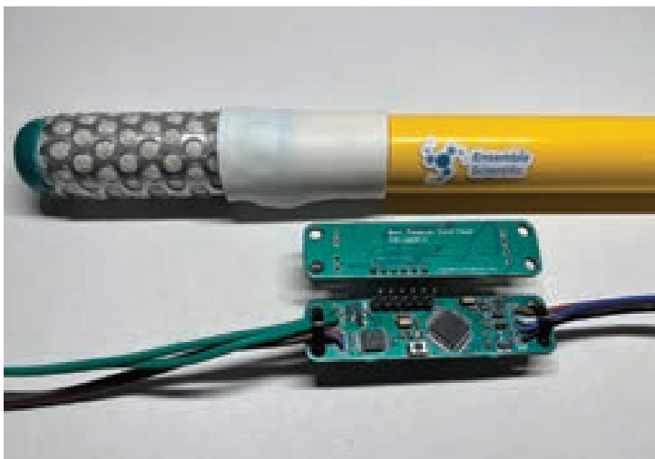
A sample of a soil tension sensor with temperature
