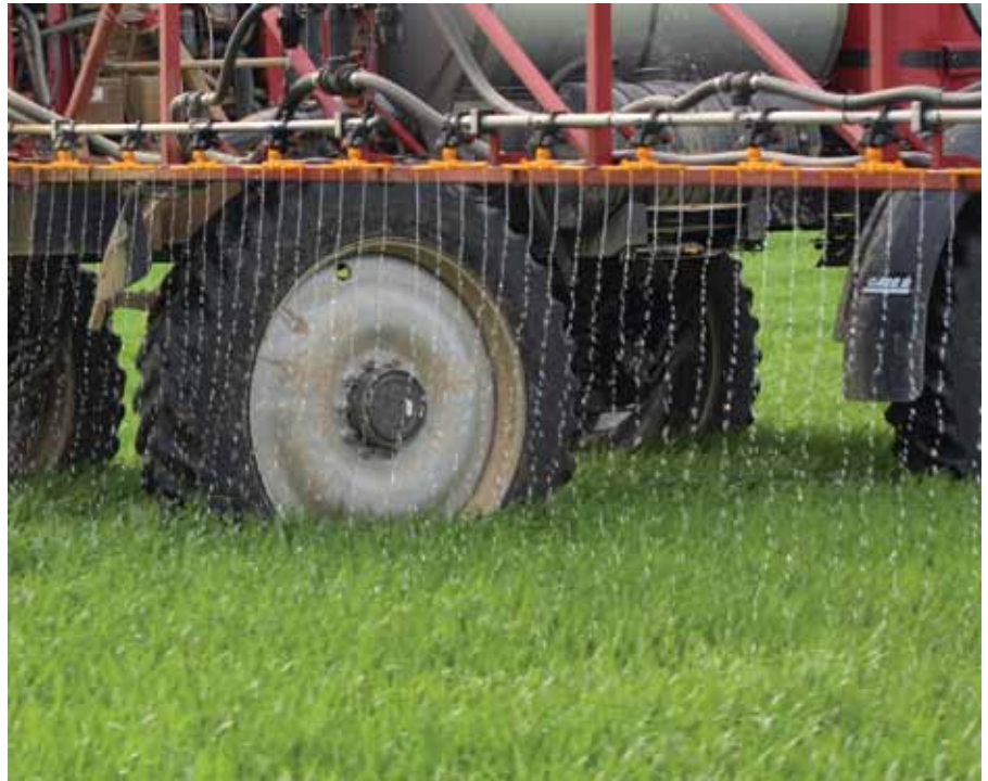
A producer uses a large self-propelled sprayer equipped with stream bars to apply liquid nitrogen. Post applications such as these are targeted to reduce risk and apply nitrogen to feed the yield potential, rather than putting all the nitrogen down at seeding time. PHOTO: PHIL NEEDHAM
